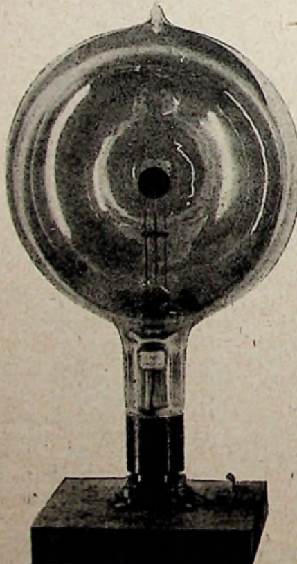
(Photo by courtesy of G.E.C., U.S.A.) A typical form of Photo-Electric Cell.
